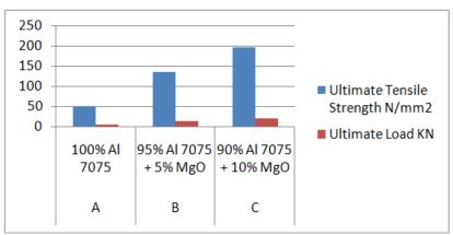
Fig:8. Graph Details of Tensile Test
