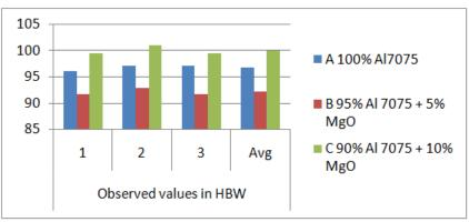
Fig:10. Graph Details of Hardness Test
